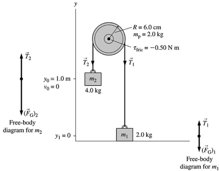
Because the pulley is not massless and frictionless, tension in the rope on both sides of the pulley is *not* the same.
